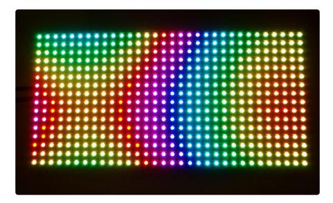
Of course, we wouldn't leave you with a datasheet and a "good luck!" We have a full wiring diagrams and working Arduino library code with examples from drawing pixels, lines, rectangles, circles and text. You'll get your color blasting within the hour! On most Arduino-compatible boards, you'll need 12 digital pins, and about 800 bytes of RAM to hold the 12-bit color image (double that for the 32x32 matrix, double again for smooth double-buffered animation).
