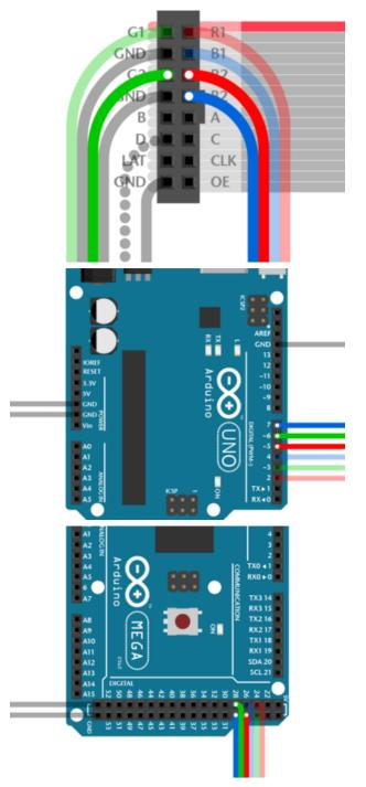
Pins R2, G2 and B2 (labeled R1, G1 and B1 on some matrices) deliver data to the bottom half of the display. These connect to the next three Arduino pins...
