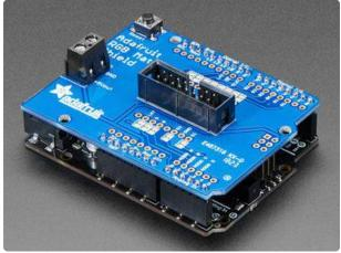
The 16-pin (8x2) header must be installed in the correct orientation! The polarity notch is indicated on the silkscreen, or you can see in the photos above that the notch faces the digital I/O pins. If you install this backwards the matrix will not work!
