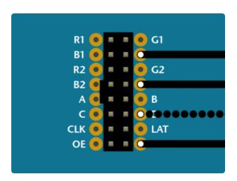
32x32 and 64x32 matrices require three ground connections. 32x16 matrices have four.
