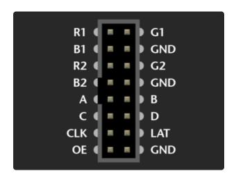
Here's the layout for 32x32 and 64x32 panels. We'll call this "Variant A." Some panels use different labels, but the functions are identical.
