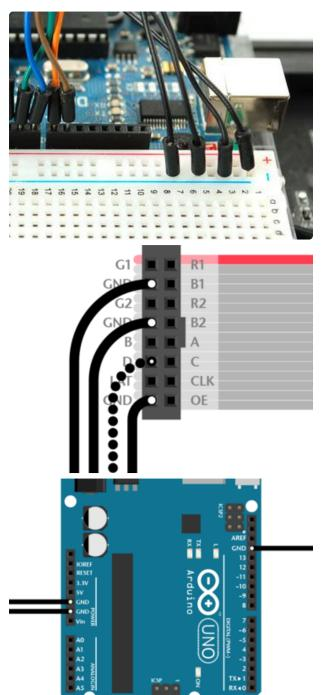
32x32 and 64x32 matrices require three ground connections. 32x16 matrices have four.
