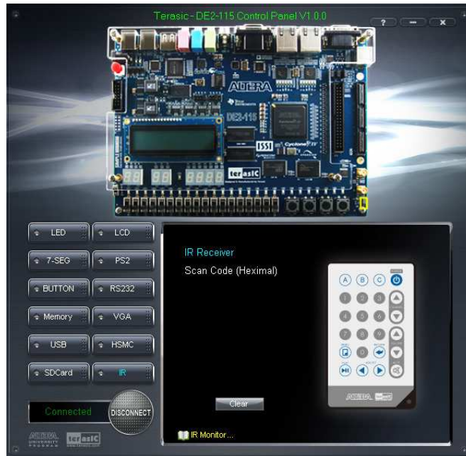
Figure 3-14 Testing the IR receiver using remote controller
