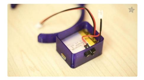
Plug the battery into the JST extender and insert the slide switch through the top opening by pressing it through the top hole of the enclosure.
