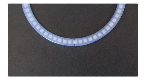
Join the two holder parts together by snapping the tabs on the ends together. Carefully insert the 60 NeoPixel ring into the assembled holder. Thread the wires through the hole of the neoring-60-bottom.stl and out the hinge connector.
