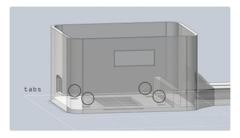
The box.stl part houses the 500mAh lipo battery and Trinket. At the bottom of the enclosure, the opening with tabs allows the connector.stl part to mount to the hotshot. stl part to the enclosure.
