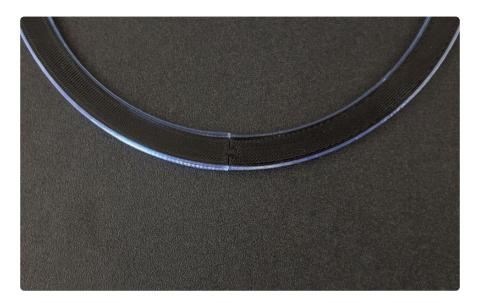
The neoring-60-top.stl and neoring-60-bottom.stl parts are the two pieces that snap together to make the large ring. The neoring-60-cap-top.stl and neoring-60-cap-bottom.stl parts are also two parts that snap together, these are to be printed in transparent PLA to diffuse the LEDs.
