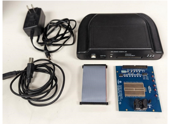
Figure 11: Connection between ASEK-20 and ACS37610 Daughterboard
