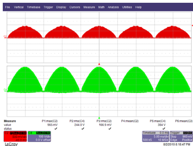
Figure 24 – 265 VAC 50 Hz, Full Load. Upper: I_{DRAIN} , 500 mA / div. Lower: V_{DRAIN} , 100 V, 5 ms / div.
