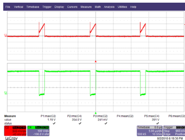
Figure 25 – 265 VAC 50 Hz, Full Load. Upper: I_{DRAIN} , 500 mA / div. Lower: V_{DRAIN} , 100 V, 5 μs / div.
