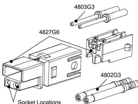
\* No extraction tool required for contact removal.
