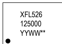
Figure 15. Marking Configuration for the 5.0 × 3.2 mm (LXG8) Package (example based on XFL526125.000000I)
