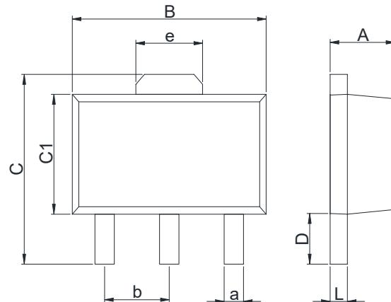
**Dimensions In Millimeters(SOT-89-3)**
