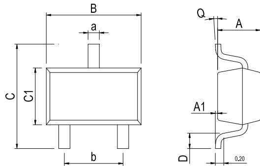
**Dimensions In Millimeters(SOT-23-3)**
