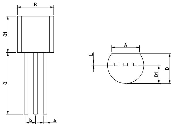
Dimensions In Millimeters(TO-92)
