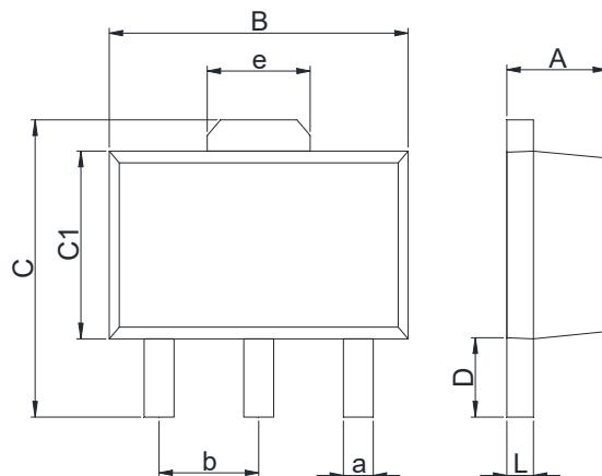
Dimensions In Millimeters(SOT-89-3)
