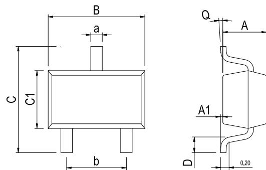
Dimensions In Millimeters(SOT-23-3)
