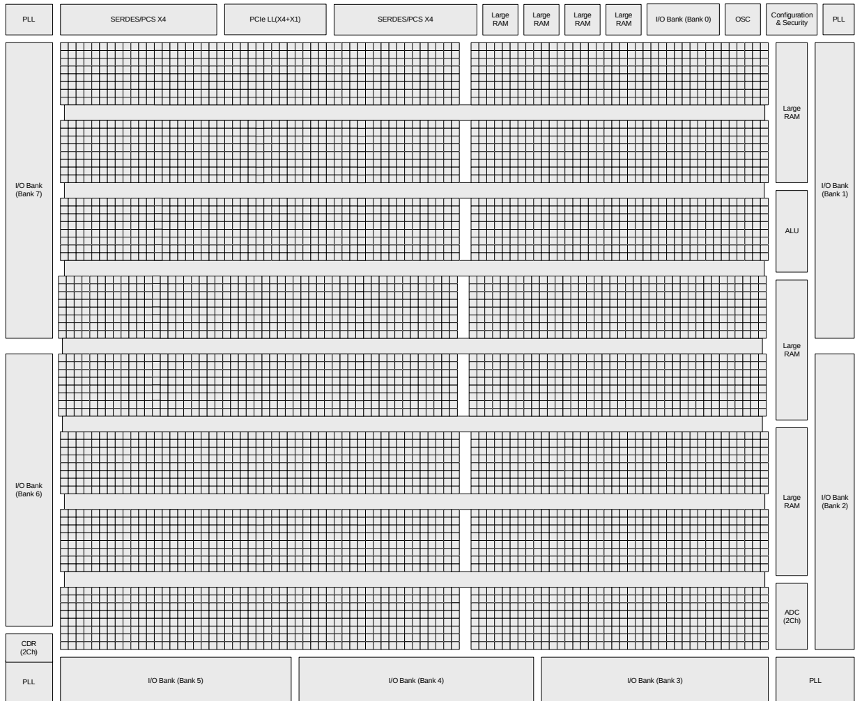
Figure 2.2. Simplified Block Diagram, LFCPNX-100 Device (Top Level)
