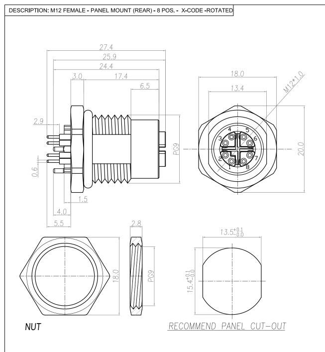
NOTE: MATERIAL HOUSING: PA UL94V-0, BLACK CONTACT: **BRASS** NUT: **BRASS** SHELL: **BRASS** □-RING: EPDM, BLACK X-SHELL: ZINC ALLOY FINISH CONTACT: GOLD 10u" MIN. **DVER 50u" NICKEL** NICKEL PLATED NUT: SHELL: NICKEL PLATED X-SHELL: NICKEL PLATED **ELECTRICAL** RATED CURRENT: 0.5A RATED VOLTAGE: 50VAC/60VDC INSULATION RESISTANCE: 100 MOhms MIN. CONTACT RESISTANCE: 10 mOhms MAX. WATER PROOF: IP67 **ENVIRONMENT OPERATION TEMPERATURE:** -40°C TD +85°C
