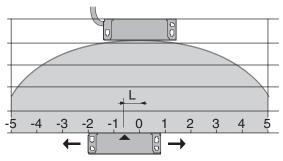
5 mm misalignment tolerance after setting
