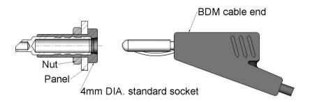
Example of a regular connection: the contact is exposed.
