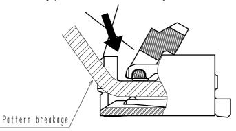
◆Checking the Locking Condition
