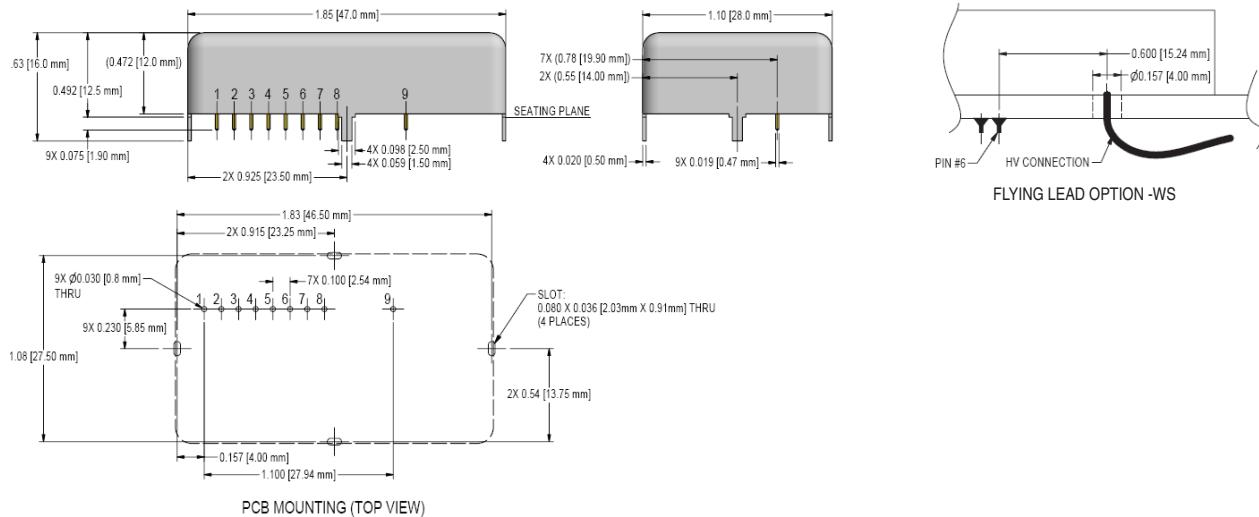
**1** Pins 7 and 8 are available for 2 k to 3 kV units with enhanced interface option ONLY.
