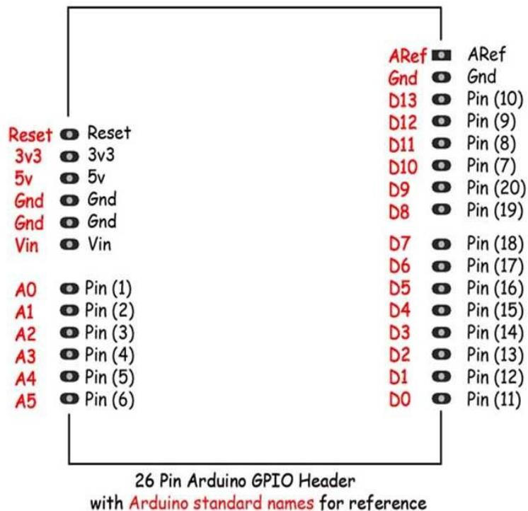
26 Pin Arduino GPIO Header
