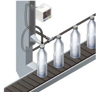
Air-leak test for PET bottles
