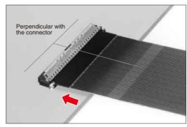
To assure correct electrical and mechanical connection do not insert FPC at angle. It must be fully inserted.
