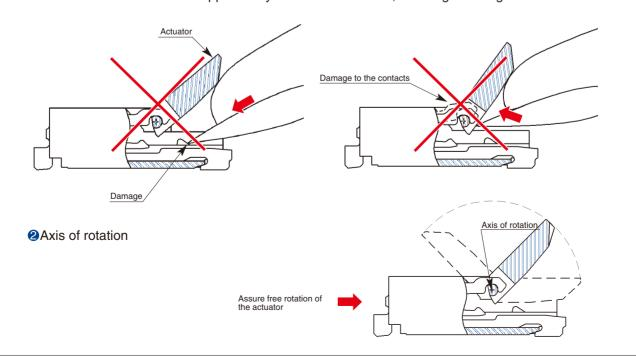
The actuator will rotate 135 degrees maximum. Do not apply force to rotate further. (1N max.)
