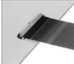
On the actuator until firmly closed. It is critical that the inserted FPC is not moved and remains fully inserted.
