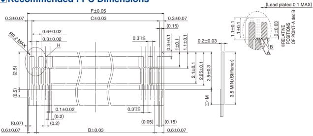
1 Dimention M must be 0.5mm minimum when the stiffener is shorter than 3.5 min.
