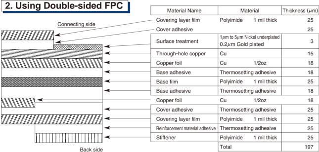
●To prevent release of the FPC due to it's bending, use of double sided FPC with copper foil on the back side is NOT RECOMMENDED.
