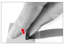
2 Fully insert the FPC in the connector parallel to mounting surface, with the exposed conductive traces facing down.
