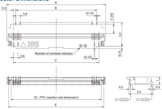
Notes 1 The coplanarity of each terminal lead within specified dimension is 0.1mm Max.
