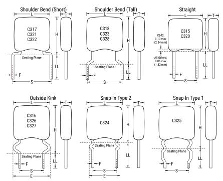
\* May be supplied in a "Shoulder Bend" or "Straight" Lead configuration. Please see Capacitance Range Waterfall section of this document to determine lead configuration availability by capacitance value.
