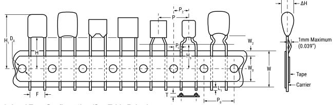
Figure 2: Lead Tape Configuration (See Table Below)
