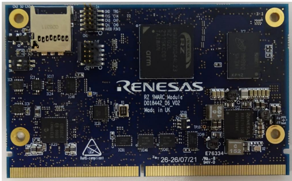
Figure 4.1 Top View of the SMARC Module Board
