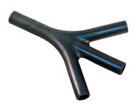
Low profile 1:3 heat shrink transitions provide an easy to install and rugged cable routing solution. Transitional boots are available in eight material options with five adhesive choices. All Adhesive lined and unlined shrink books are RoHS compliant. Transitional boots are water-tight when equipped with factory installed or user-installed adhesive. Choose boot size based on cable diameter.
