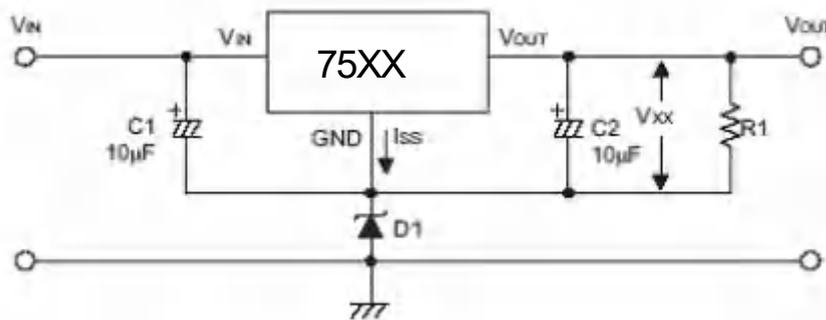
$$V_{OUT} = V_{XX} + VD1$$
