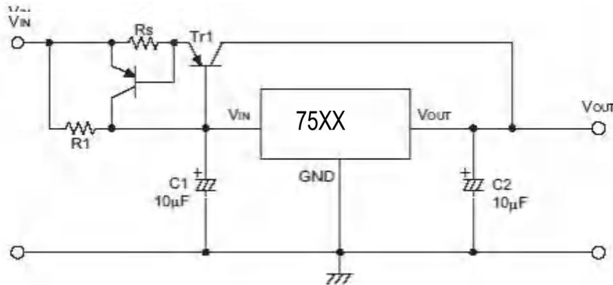
4. Circuit for increasing output voltage (1)
