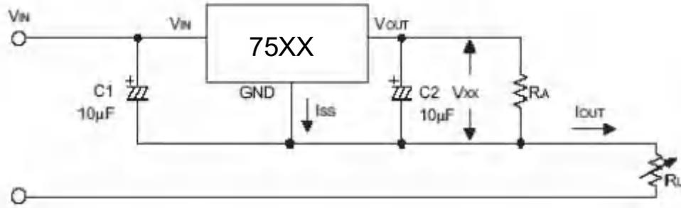
$$I_{OUT} = V_{XX}/R_X + I_{SS}$$
