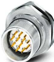
M23, Device connector rear mounting, series: CA, straight, shielded: yes, for standard and SPEEDCON interlock, No. of pos.: 12, Direction of rotation: Standard, contact connection type: Pin, Solder connection, Axial seal, Central fixing, coding: N, Alternative product in accordance with RoHS II without Exemption 6c (Pb < 0.1 %) item no.: 1243841
