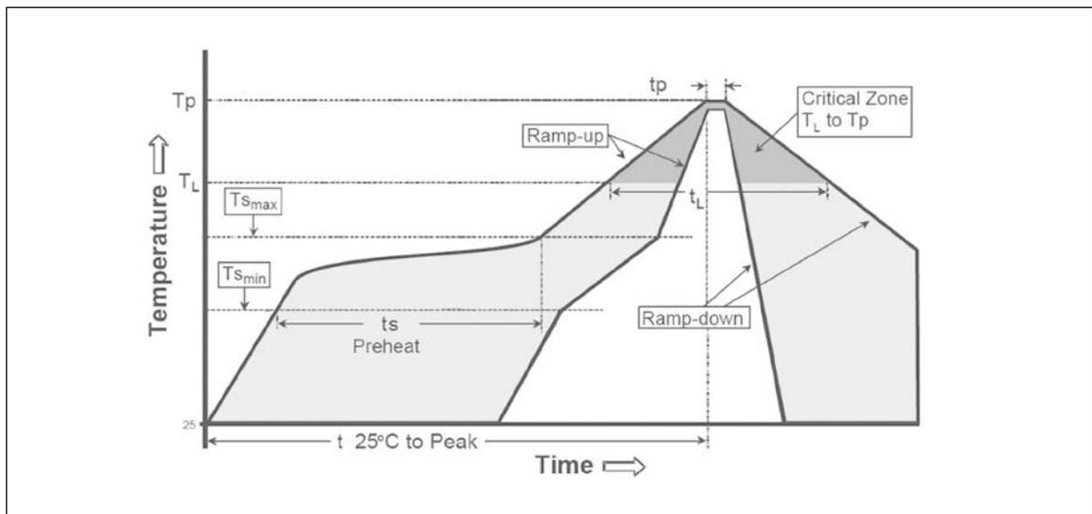
The detailed settings for the reflow profile can be derived from this table.
