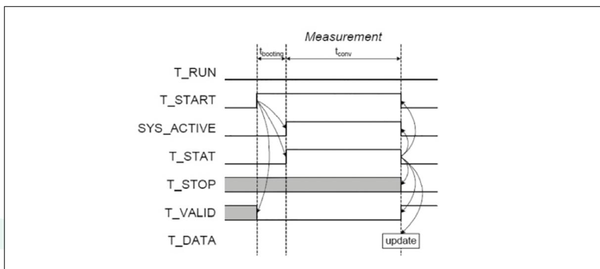
Signal T\_RUN is written low to select a single shot measurement. Note that T\_STOP is typically low (cleared by a previous measurement), but its state is ignored in a single shot measurement. T\_START is written high to start measuring: T\_VALID in T\_VAL is cleared and the device starts *booting* to *active*. Once active SYS\_ACTIVE goes high, and measurement starts (T\_STAT goes high).
