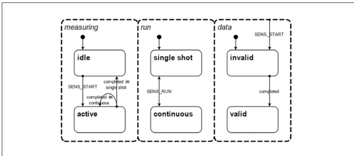
When in the *single shot* run mode, starting a measurement is under control of the master. By default a sensor is idle; it can be started by writing a 1 to the corresponding bit in SENS\_START. After a start, the sensor stops when the measurement is completed. Whether a sensor is idle or active measuring can be detected by reading SENS\_STAT. The measured values can be obtained via their respective readout registers (T\_VAL and H\_VAL). Writing to SENS\_STOP in single shot has no effect.
