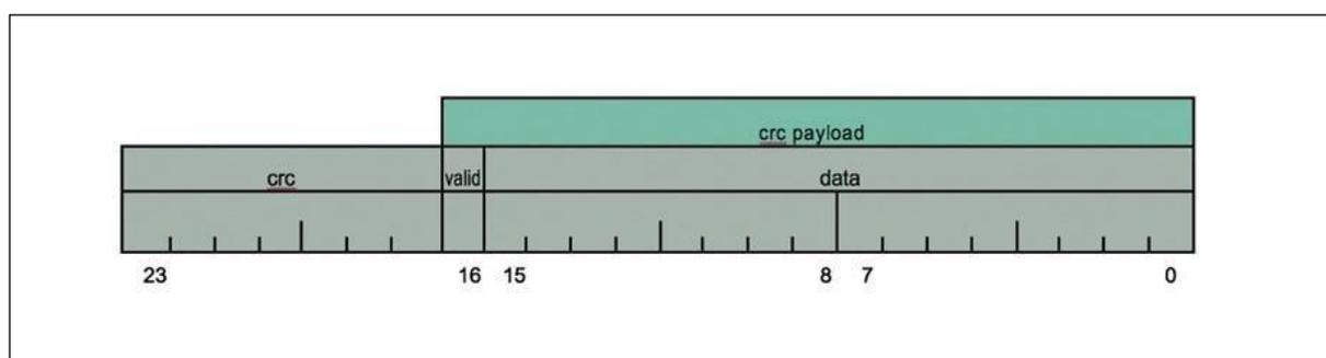
The *checksum* is a cyclic redundancy check over the data and the valid flag; the stored checksum is the result of CRC-7 (polynomial  $x^7+x^3+1$ , see [https://en.wikipedia.org/wiki/Cyclic\\_redundancy\\_check](https://en.wikipedia.org/wiki/Cyclic_redundancy_check)) with 0x7F as initial vector (*i.e. with all bits flipped*), see [Computing CRC-7](#) for sample C code.
