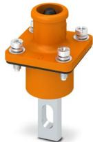
Connector, Range of articles: BPC, color: orange, number of positions: 1, min. conductor cross section: 35 mm<sup>2</sup>, max. conductor cross section: 70 mm<sup>2</sup>, rated voltage: 1500, rated current: 250 A, Connection method: Screw/Solder connection, Contact connection type: Pin
