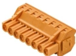
Clamping-yoke connection with right-angled (90° or 270°) or angled (225°) outlet direction. The female connectors provide space for labelling and can be coded. Fastened by means of a flange or release latch. They also provide an integrated plus/minus screw, protection against faulty insertion of the wire, and they are delivered with open clamping yokes. HC = High Current.
