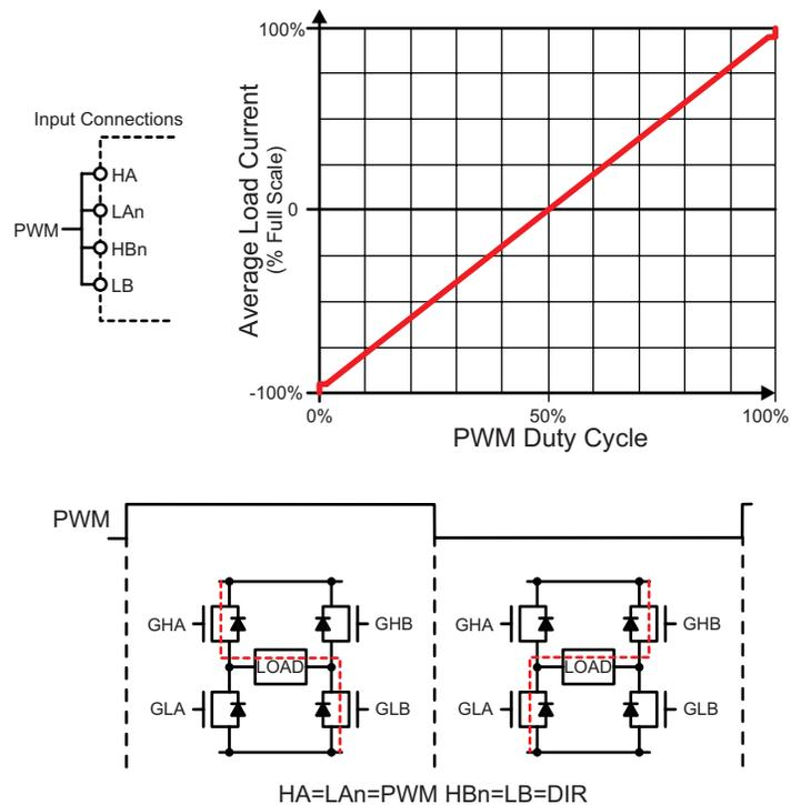
Figure 9: Single PWM Input, Fast Decay, SR
