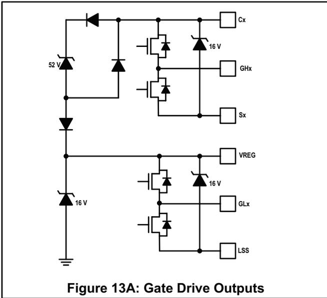
Figure 13A: Gate Drive Outputs
