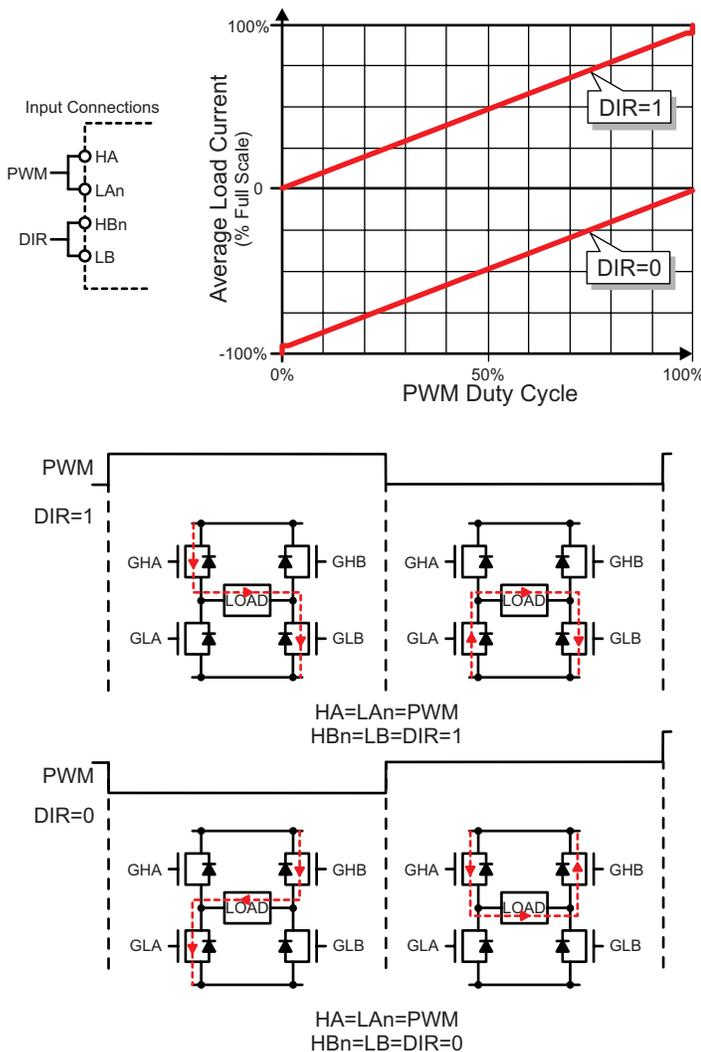
Figure 8: PWM and DIR Inputs, Slow Decay, SR
