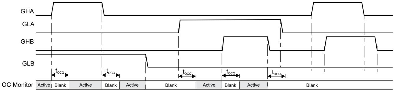
Figure 4: Overcurrent Fault Monitor – Blank Mode Timing (OCQ = 1)
