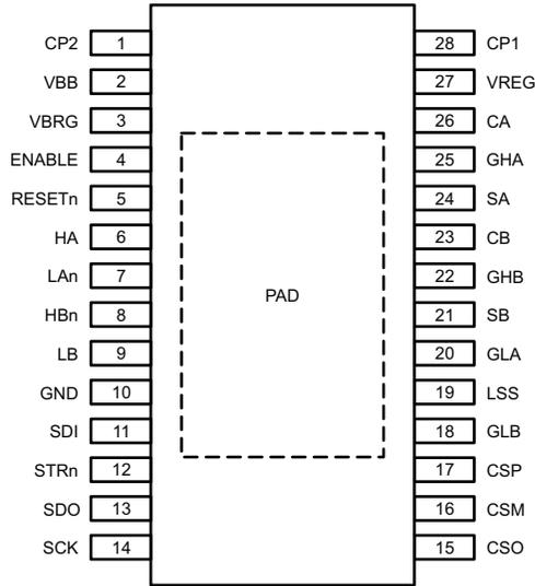
Package LP, 28-Pin eTSSOP Pinout Diagram
