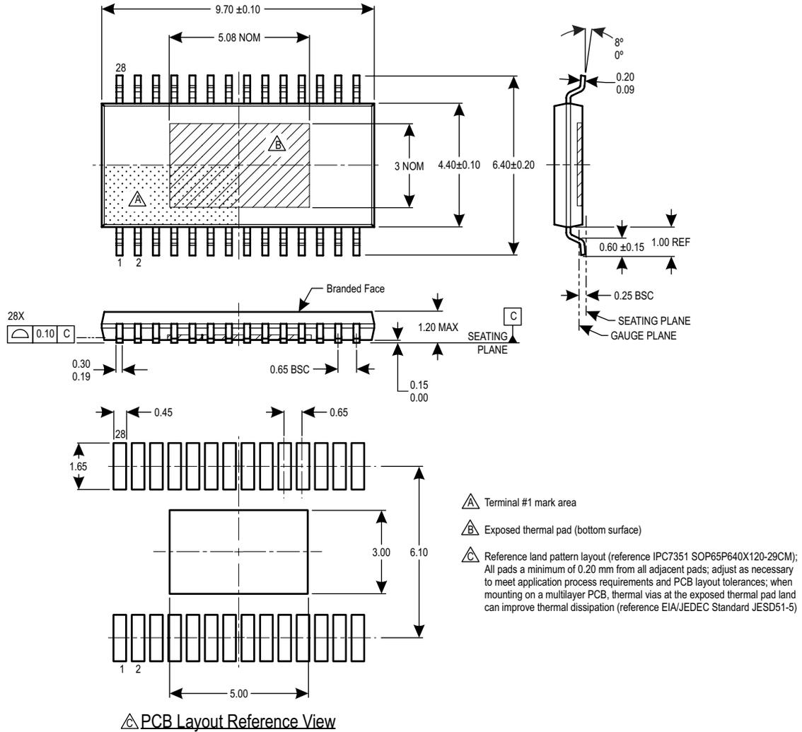
Figure 14: Package LP, 28-Pin eTSSOP with Exposed Pad
