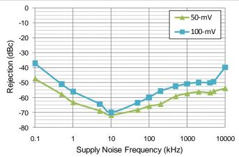
Power supply rejection ratio
