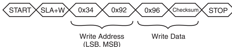
FIGURE 8-2: EXAMPLE OF A WRITE TO ADDRESS 0x1234 WITH A CHECKSUM
