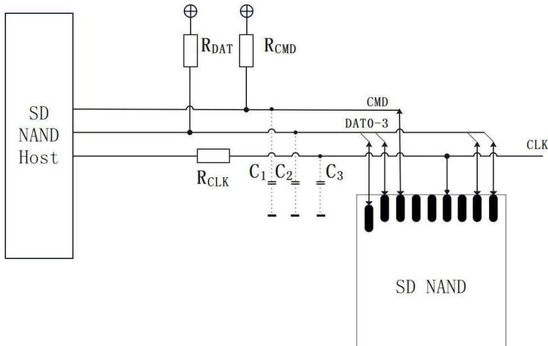
RDAT and RCMD (10K~100 kΩ) are pull-up resistors protecting the CMD and the DAT lines against bus floating when Nano SD NAND is in a high-impedance mode.
