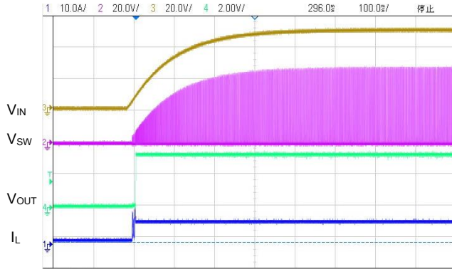
(19) Power Ramp Up (VIN=50.0V, VOUT=3.3V, IOUT=0.6A)
