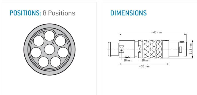
The pin layout corresponds to the view on the termination area
