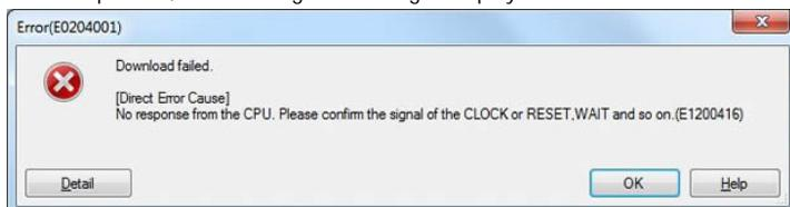
In order to avoid this error, open the RL78 E1 (Serial) Property, and set the "Erase flash ROM when starting" on the Connect Settings tab to YES, to download the program.
