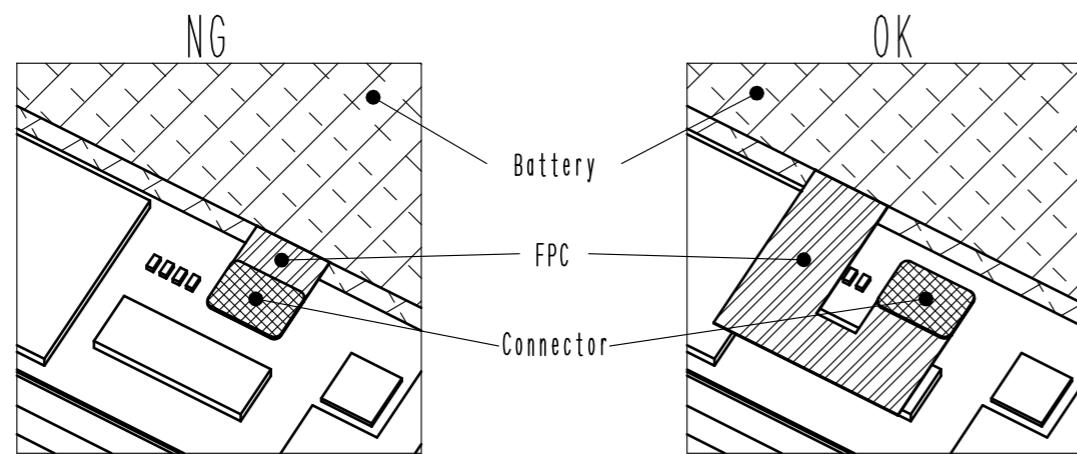
\*Possible problems caused by connector mating in incorrect positioning.
