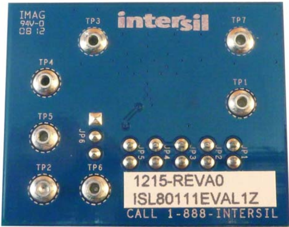
FIGURE 2. ISL80111EVAL1Z BOTTOM SIDE
