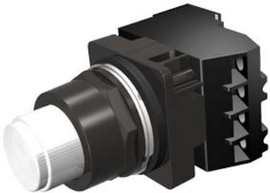
30mm BlackMax, Epoxy Coated Corrosion Resistant Complete Metal Unit PTT / Illuminated Pushbutton Transformer type, 120V AC Incandescent Lamp Extended Button Plastic Lens, White 2 Position Momentary with 1 N.O. - 1 N.C. Heavy Duty Contacts, A600/P600 UL Listed, CSA Certified NEMA 1,3,3R,4,4X,12,13 & Automotive Standards
