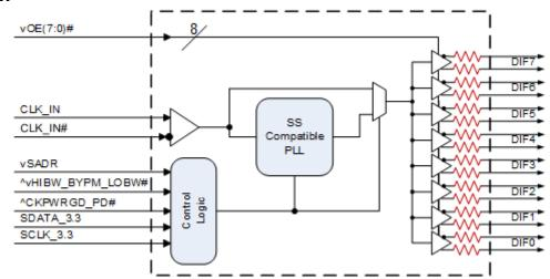
Note: Resistors default to internal on 41/51 devices. P1 devices have programmable default impedances on an output-by-output basis.
