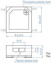
The positive polarity terminal: 1 The negative polarity terminal: 2=3=4 common Dimensions in mm
