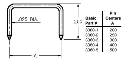
Description: 3360 - Jumper Pin Packaging: Packaged in Bulk
