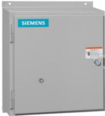
Non-reversing motor starter, Size 2, Three phase full voltage, Solid-state overload relay, OLRelay amp range 13-52a, 208VAC 60HZ coil, Non-combination type, Enclosure type 12, Dust/drip proof for indoors, Extra-wide enclosure
