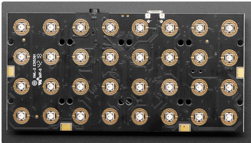
The NeoPixels are chained together, and connect in a zig-zag. The first pixel is in the top left, the last pixel is on the bottom right. In Arduino, the NeoPixels are on pin 10, in CircuitPython they are on `board.NEOPixel`
