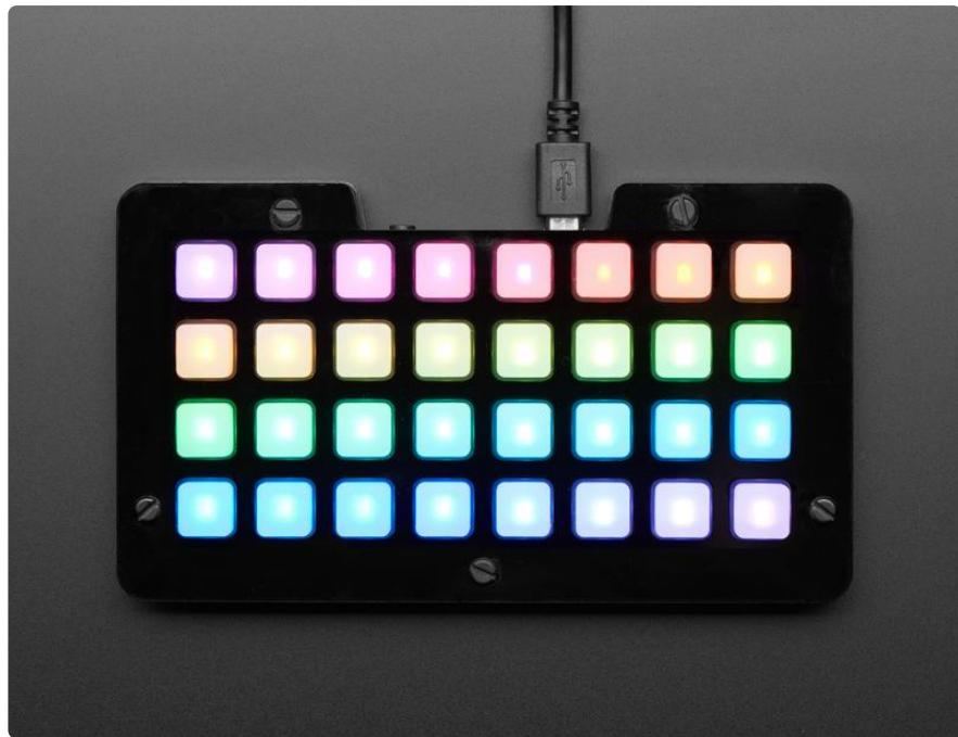
Time to make some noise! We picked the SAMD51 mostly because its got that dual DAC - that's two 12-bit, 500KSPS 'true analog' outputs and we connected them to left and right on a standard headphone jack. Since the DAC pins are also ADC pins you could also use the left/right for audio line level input if you so choose. You're not going to get audiophile-quality outputs from two 12-bit DACs but you can certainly play audio clips and make beeps and bleeps.
