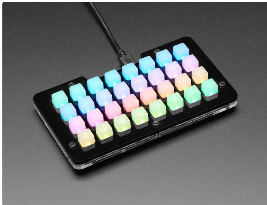
The NeoTrellis M4 is an all-in-one USB + NeoPixel + Elastomer + Audio board. It's powered by our new favorite chip-in-the-world, the SAMD51, a Cortex M4 core running at 120 MHz. This chip has a speedy core with CircuitPython and Arduino support, hardware DSP/floating point, dual DACs (more on that later!) and all the
