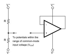
**Remark**: A midpoint potential of V<sup>+</sup> and V<sup>-</sup> is applied to this example.
