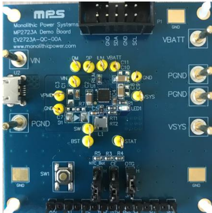
Figure 2: EV2723A-QC-00A Evaluation Board
