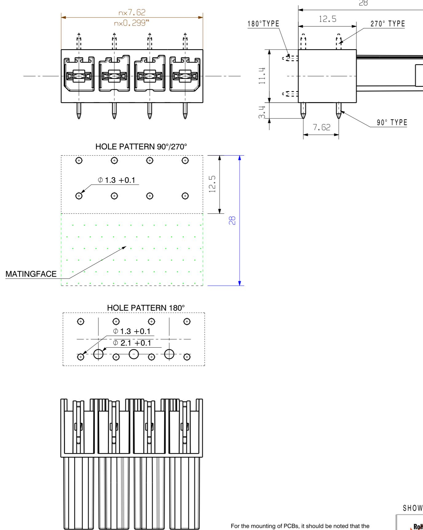
For the mounting of PCBs, it should be noted that the rated data given in the catalogue relates only to the connection elements. The necessary creepage and clearance paths must be observed in connection with the respective applicant in accordance to VDE 0110. The current-carrying capacity and pitch tolerance is to be determined according to DIN IEC 326 part 3 very fine.
