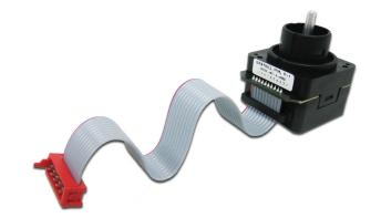
The 60C is a cost-effective replacement of a stationary mouse or trackball with improved control over cursor movement. An integral Schmitt Trigger is used to stabilize against noise and vibration.
