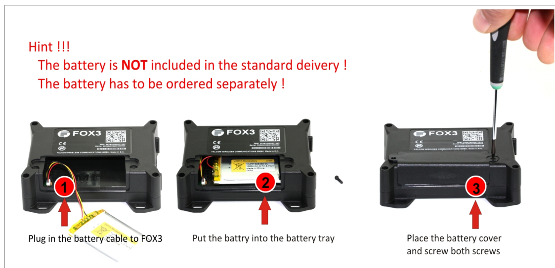
Figure 14.1: Connecting the battery to the FOX3-2G/3G/4G devices
