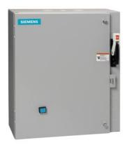
2-speed 3-phase motor starter Size 0 One winding consequent pole Constant or variable torque Solid-state overload relays Low SPD OLR range 0.25-1A High SPD OLR range 5.5-22A 110V 50HZ / 120V 60HZ coil Combination type 25Amp circuit breaker Enclosure NEMA type 4/12 Water/dust tight for outdoors
