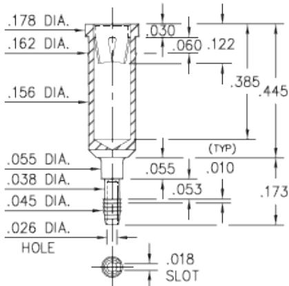
**8963-0-31-XX-08-XX-04-0**Compliant press-fit in  $.040 \pm .003$  plated hole. For  $.060 \rightarrow .100$  thick board.**Description:**
