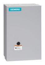
2-speed 3-phase motor starter Size 3 Two separate windings Constant or variable torque Solid-state overload relays Low SPD OLR range 25-100A High SPD OLR range 25-100A 110-120/220-240VAC 60HZ coil Enclosure NEMA type 1 Indoor general purpose use
