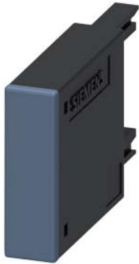
surge suppressor, varistor, 24-48 V AC, 50/60 Hz, 24-70 V DC, for contactors 3RT2.1 and auxiliary contactors 3RH2, multi-unit packaging, pack = 10 units
